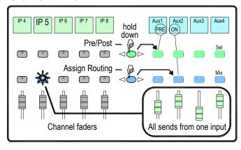
Press an Input Channel strip Mix key.
