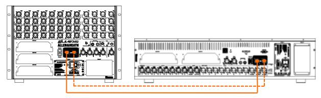
Switch on the MixRack first, then the Surface. The gigaACE Lnk/Err indicators flash at a steady rate when the link is established. The red error indicator lights if a communication error is detected. Check that the cables are correctly plugged in and are not faulty.
