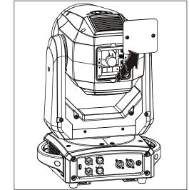
Loosen the screw in the recess.
