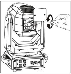
Lift the lamp out of its recess, disconnect the lamp and replace it with a new Philips MSD Platinum 12 R LL lamp..
