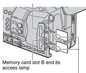
Insert with the notched corner first, and facing down.
