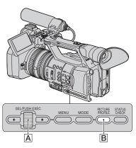
You can customize the picture quality by adjusting picture profile items such as [GAMMA] and [DETAIL].
