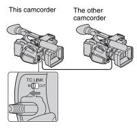
The time code of this camcorder synchronizes with that of the connected camcorder. [TC IN] appears on this camcorder screen.
