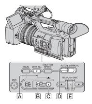
You can adjust and fix the white balance according to the lighting conditions of recording environment.
