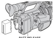
BATT RELEASE (battery release) button
