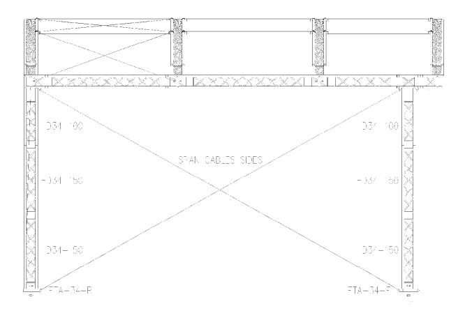
The FD34/HD34 small bases are in 2 variants. The front legs are fitted with 2 cable attachment plates inline. They are fitted so that the plates are on the outside of the roof. The rear legs have 2 cable attachments in a 90° corner. These are fitted so that 1 plate points to the front, and 1 plate is in the rear plane.
