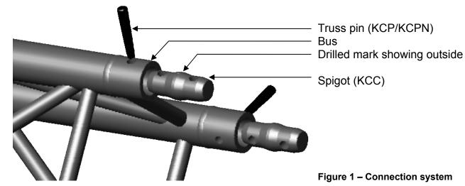
To connect 2 pieces of truss together, spigots are inserted in one truss. Insert the spigot with the drill mark on the outside. Spigots are fastened by truss pins that are hammered through the bus and the spigot. A correctly mounted truss pin is hammered so far in that the r-spring can easily be mounted or in case of a KCPN type truss pin until the entire length of the thread sticks out on the inside of the truss.
