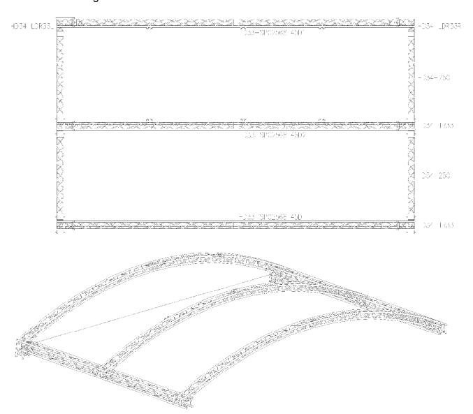
Attach HD34 139,5cm trusses to the third arc and add an HD34-TR (roof t-joint). Build the front arc. Use HD34-L90R33L and HD34-L90R33R to connect the arc to the rig.
