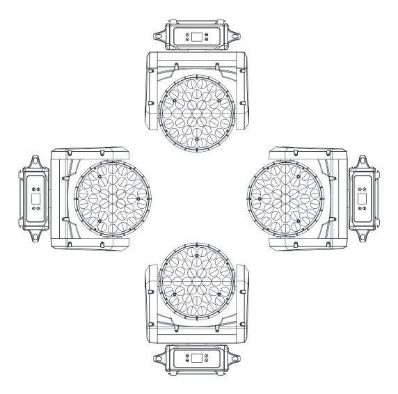
The Vizi Wash Z37 is fully operational in three different mounting positions, hanging upside-down, mounted sideways on trussing, or set on a flat level surface. Be sure this fixture is kept at least 12m (40ft) away from any flammable materials (decoration etc.). Always use and install the supplied safety cable as a safety measure to prevent accidental damage and/or injury in the event the clamp fails (see next page). Never use the carrying handles for secondary attachment.
